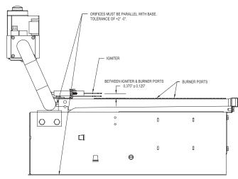
Figure 29. Igniter position to burners.
